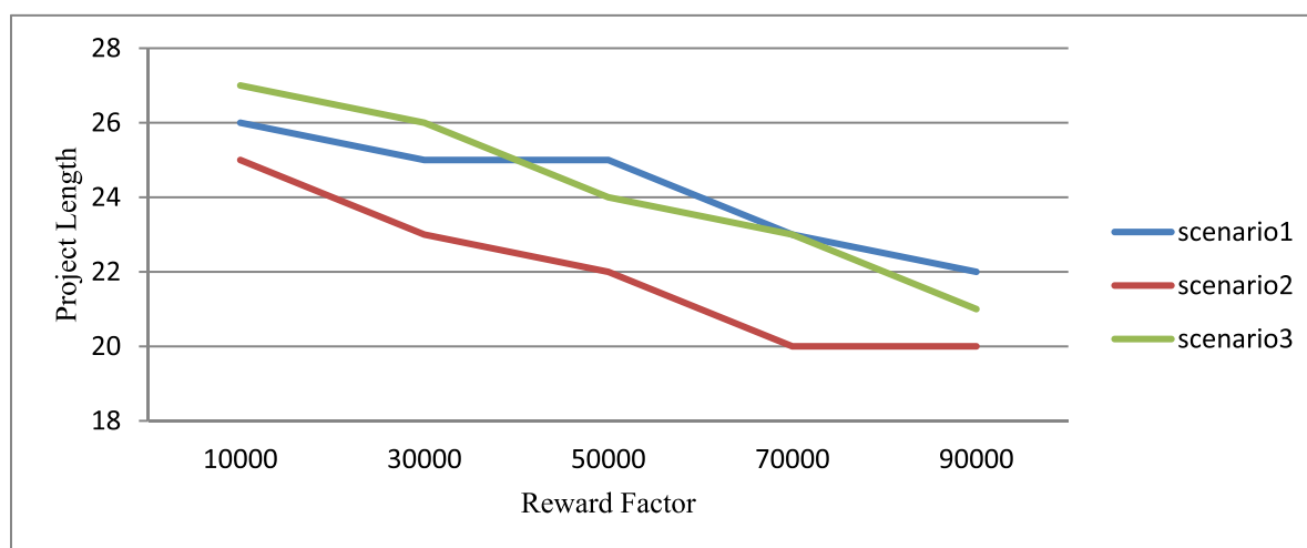
Fig. 13. Effects of early-completion reward factor on the project length.
