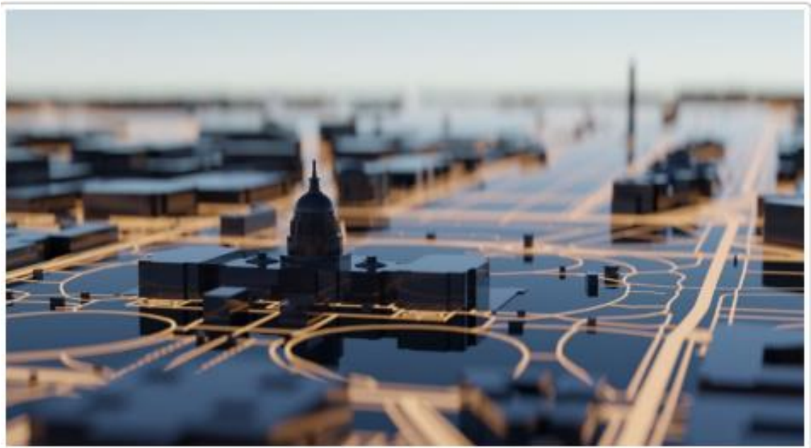
Figure: A digital twin 3D model of a city, used to simulate various climate intervention scenarios (e.g., testing where adding green roofs or floodwater storage would be most effective in reducing future risks). Such virtual city models allow planners to experiment with different strategies before implementing them in the real world.
