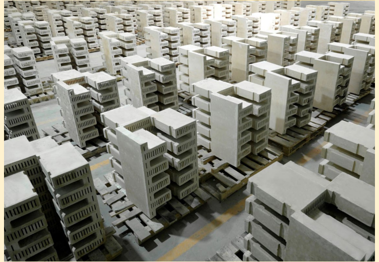
Rondo Energy uses refractory bricks to store heat
