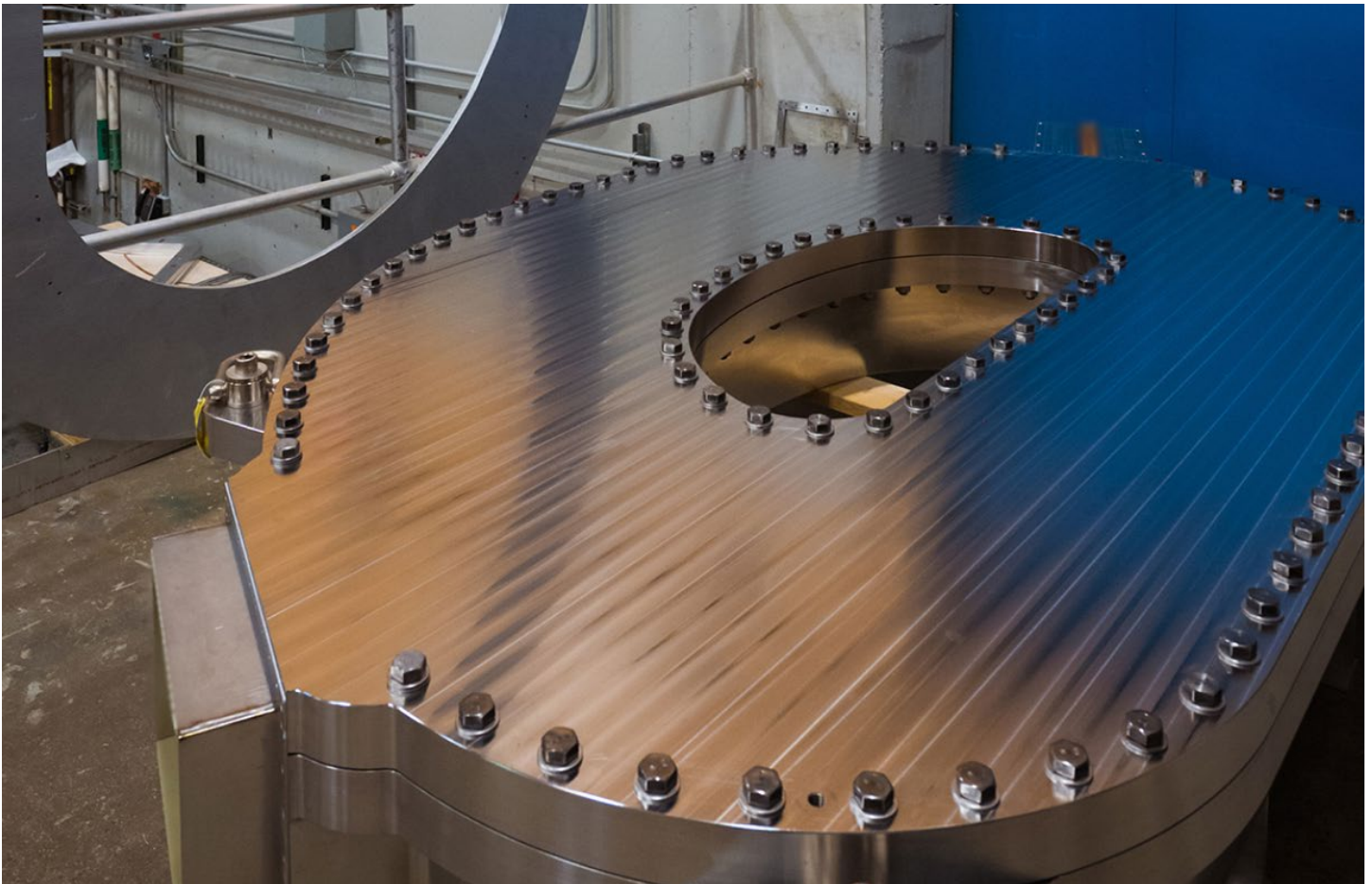
High temperature superconducting (HTS) magnet developed by Commonwealth Fusion Systems
