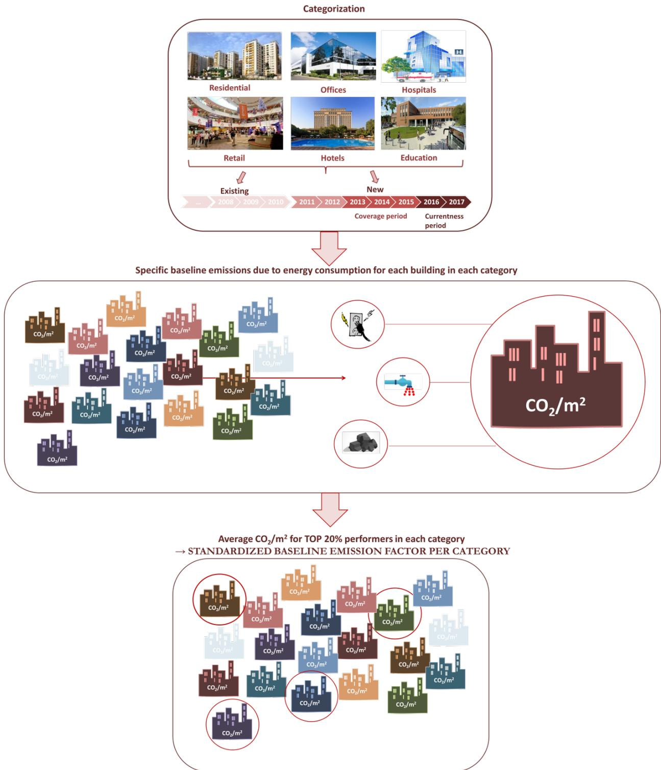
**Figure 3-2: Overview of methodology for standardized baseline emission factor determination**
