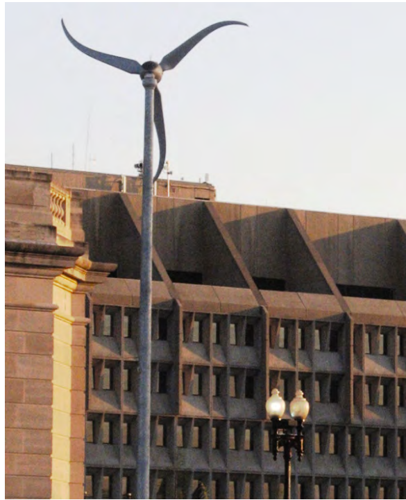
Figure 4.13.1: Horizontal axis wind turbine (HAWT)
