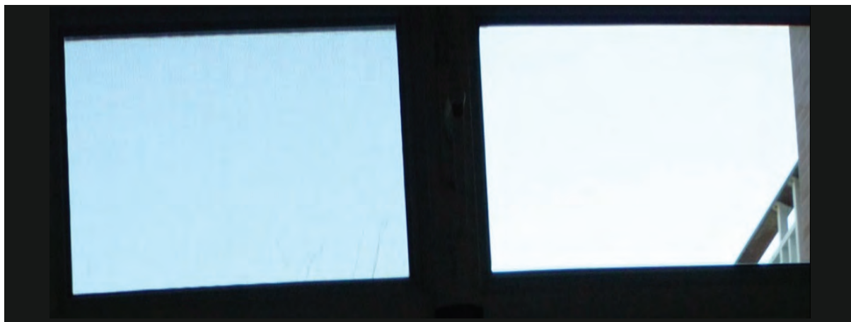
Figure 4.5.5: Photochromic glass (left) and clear glass (right) in a bright daylight environment
