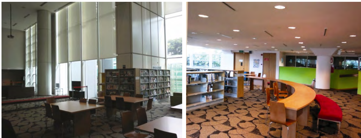
Figure 4.8.4: Zone control allows the library space near the window tapping on daylight (left), while the space away from the window is illuminated by CFLs
