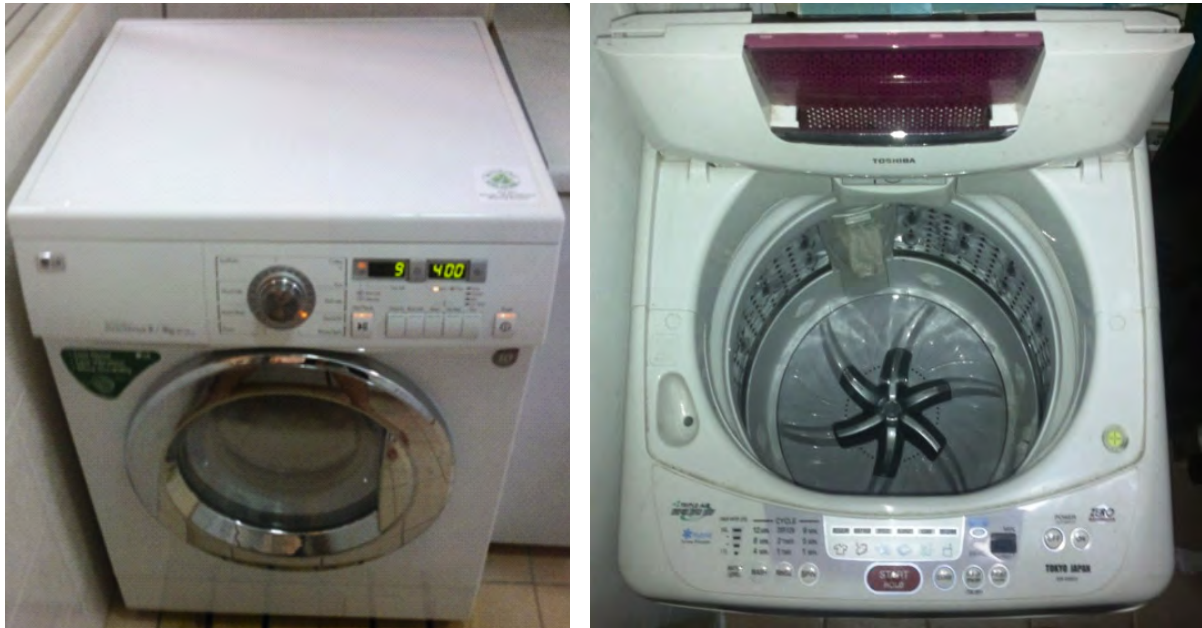
Figure 4.9.5: Water saving front-end washer (left) and conventional top-loading washer (right)
