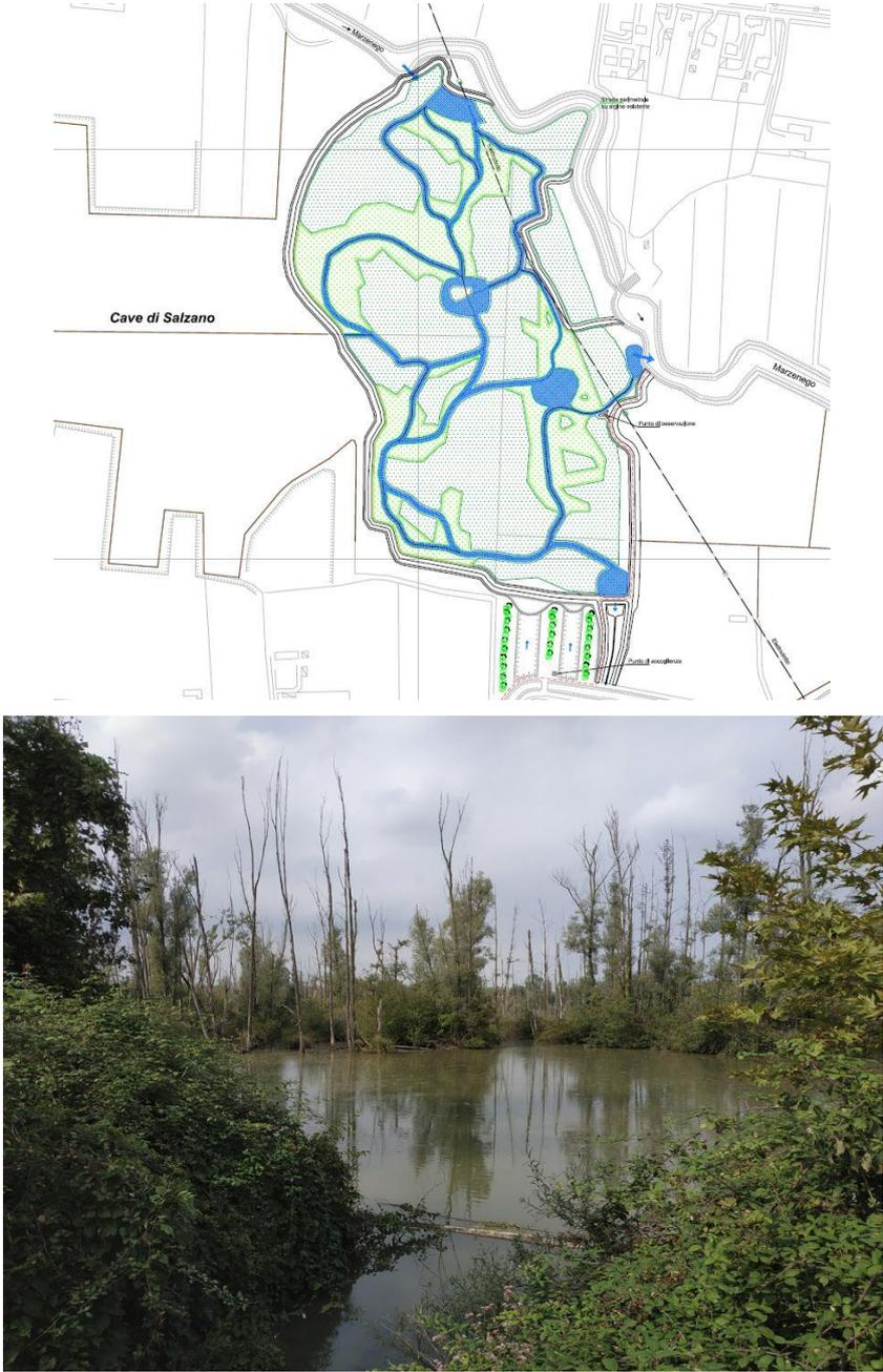
**Figure 8.** Above: plan view of the Salzano wetland, built within the Salzano quarry: wood area (dark green dots); vegetated free water surface (FWS) area (light green dots); open water FWS area in blue. Below: a view of the wetland.
