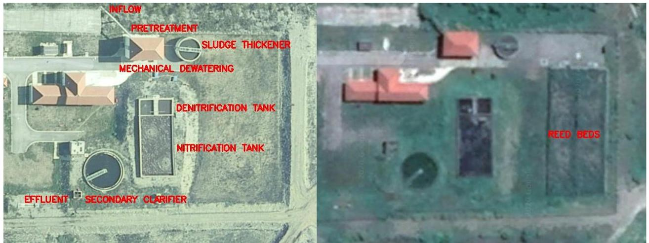
**Figure 5.** Aerial picture of Mojkovac WWTP before (left) and after RBs installation (right), from Google Maps™.
