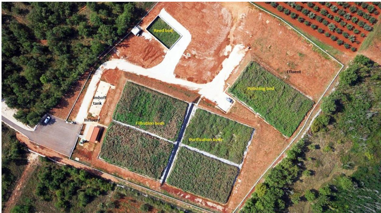
**Figure 4.** Aerial picture of the Kastelir WWTP, with indication of the treatment stages.
