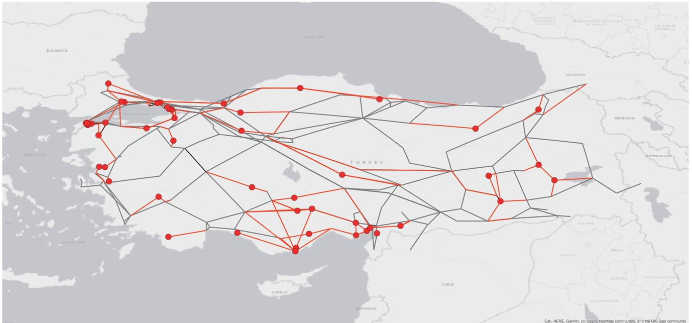
It is worth highlighting that there is a considerable investment in the 400-kV grid even for a lower base demand projection (360 TWh, Table 2). This facilitates the integration of new generation and demand as will be seen in the network simulation results, including the required redispatch and RES generation curtailment.
