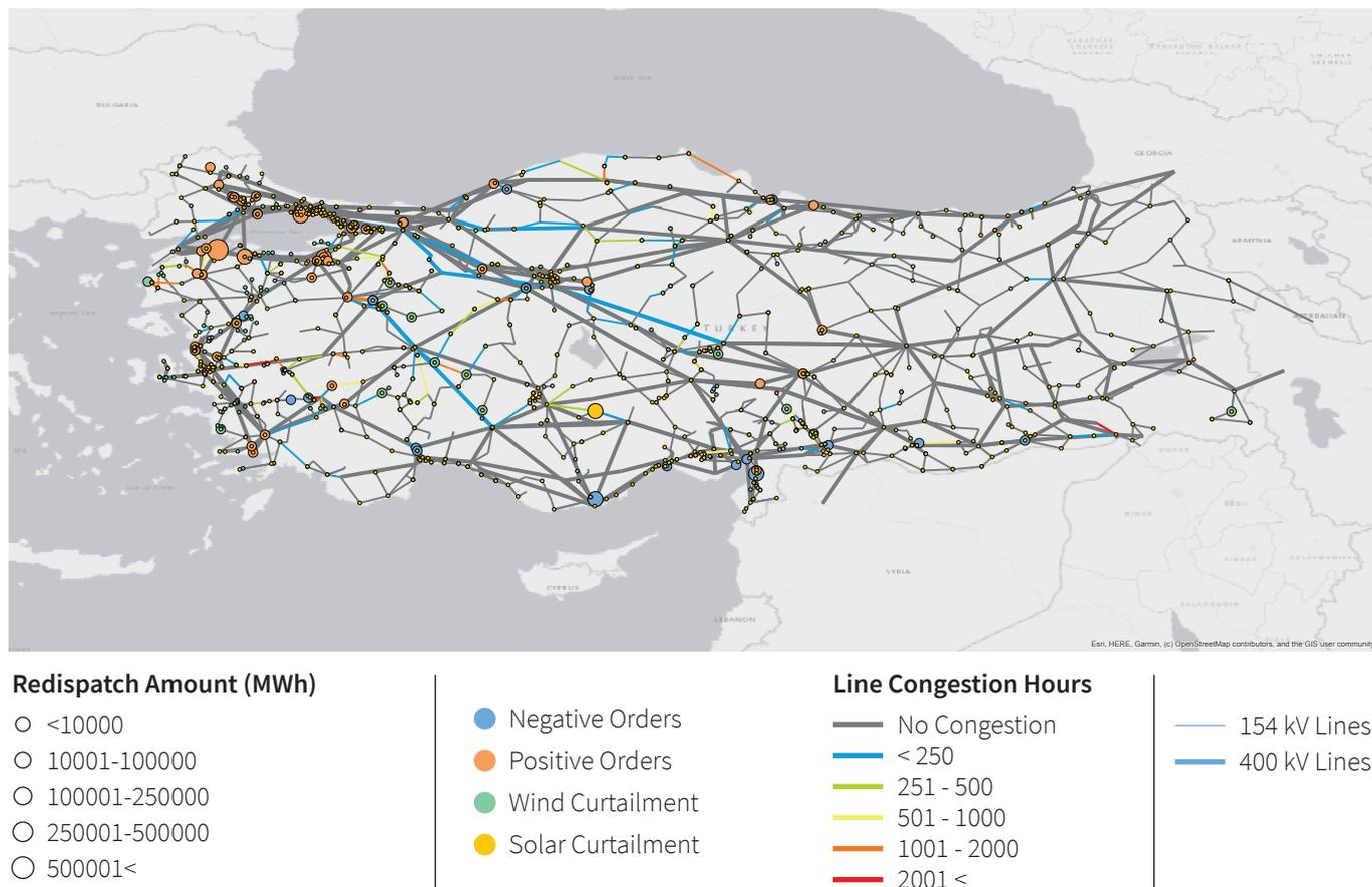
Figure 55: ARES - More Flex results (400 kV and 154-kV)
