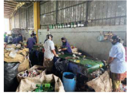
3. Primary sorting at the conveyor belt
